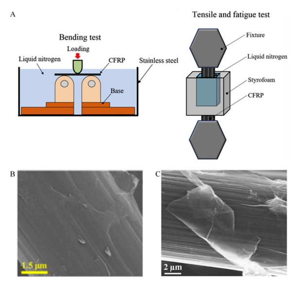
**Figure 2.** (**A**) Schematic diagrams of cryogenic testing system for three-point bending and tensile tests. Reprinted from ref. [106], Copyright 1969 Elsevier Ltd. (**B**) SEM image of GO coated SCFs. Reprinted with permission from ref. [105], Copyright 2016 Elsevier Ltd. (**C**) SEM images of graphene oxide grafted on CF. Reprinted with permission from ref. [107], Copyright 2020 Elsevier Ltd.
