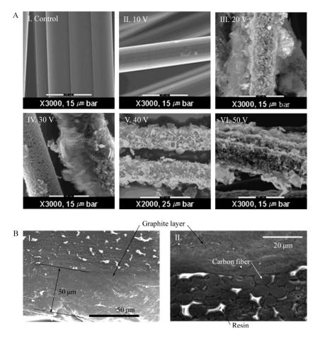
**Figure 4.** (**A**) SEM images for the surface of CFs at different applied voltages for 5 min. Reprinted with permission from ref. [112], Copyright 2008 Elsevier Ltd. (**B**) SEM images: I. composite plate coated with a 2-µm-thick graphite layer; II. composite plate coated with a 50-µm-thick graphite layer. Reprinted with permission from ref. [116], Copyright 2011 Elsevier B.V.
