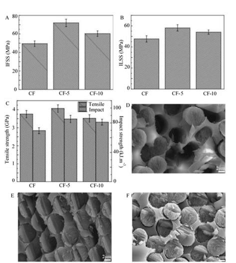
**Figure 3.** Mechanical properties of carbon black coated CFs/epoxy composites: (**A**) IFSS tests results of the composites. (**B**) ILSS of the composites. (**C**) Impact test results of the composites and single fibre tensile strength. SEM morphologies of the fracture surface of composites (**D**) the untreated-CF, (**E**) CF-5 min, (**F**) CF-10 min. Reprinted with permission from ref. [22], Copyright 2017 Elsevier Ltd.
