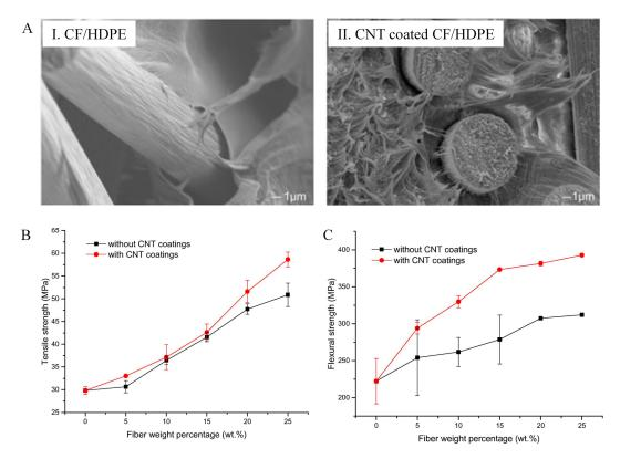
**Figure 7.** Effect of CNT coating on morphological and mechanical properties of CF reinforced HDPE composites: (**A**) Fracture morphologies: I. Neat CF/HDPE composite; II. CNT coated CF/HDPE composite. (**B**) Comparison of tensile strength. (**C**) Comparison of flexural properties. Reprinted with permission from ref. [32], Copyright 2019 Elsevier Ltd.
