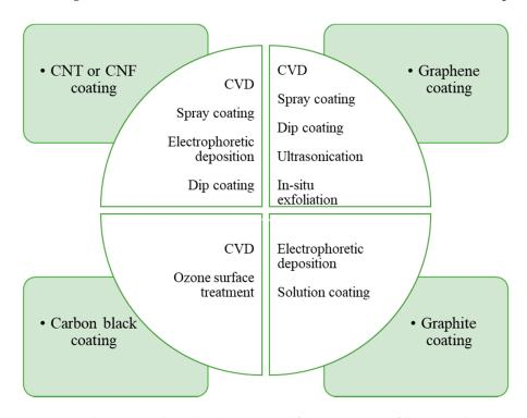
Figure 8. Carbon materials and techniques used for CF coating to fabricate polymer composites.
