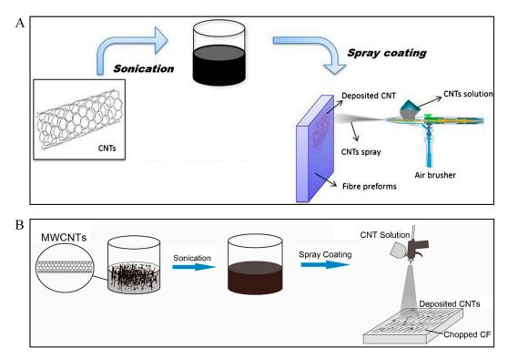
**Figure 6.** Schematic illustrations of CNT spray coating. (A) Onto CF prepreg. Reprinted with permission from ref. [121], Copyright 2014 Elsevier Ltd. (B) Onto chopped CFs. Reprinted with permission from ref. [32], Copyright 2019 Elsevier Ltd.
