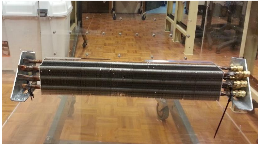
Figure 5.20: Finned type cross-flow in-line heat-pipes -heat-exchanger with R134a as the cooling medium.
