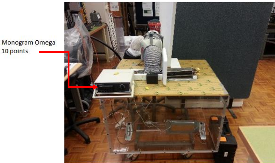
Figure 4.29: The 10 terminal point data logger for data collections. The main purpose is to measure the outside ambient air temperature and compared it to the processed data recorded in the acrylic box.
