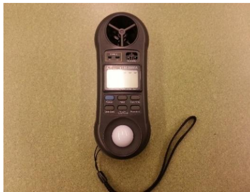
Figure 4.31: A Lutron LM-8000A Type K anemometer collects the velocity and the temperature.
