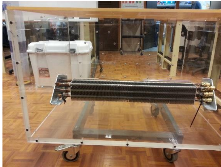
Figure 4.26: An acrylic box with the heat-pipes heat-exchanger attached to the sidewall. The opening is created to let the air pass through the inlet and outlet.
