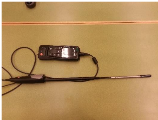
Figure 4.32: A Testo Hot-wire Anemometer record the velocity and the temperature inside the acrylic box.
