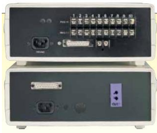
Figure 4.34: A Monogram Omega data logger with a 10-point terminal to record the temperature.
