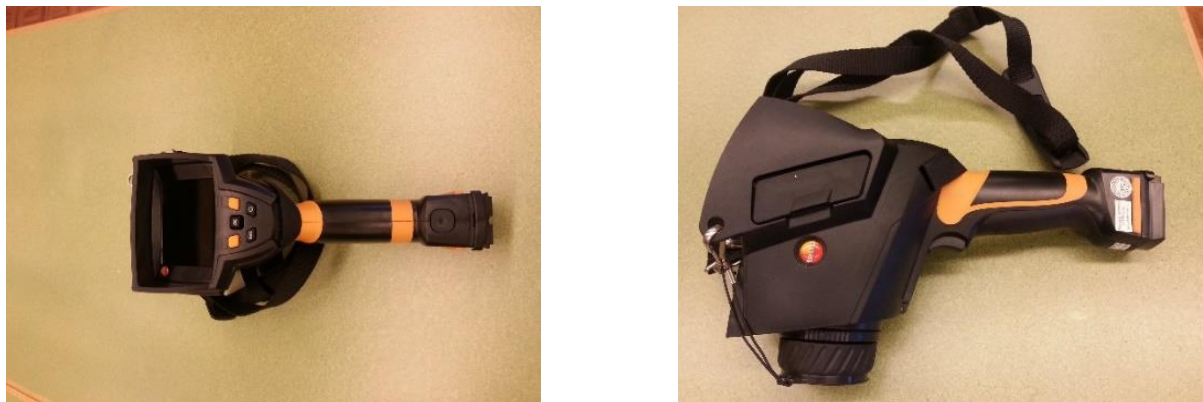
Figure 4.33: A Testo Thermal-Image 875 for digital imaging of temperature distribution.
