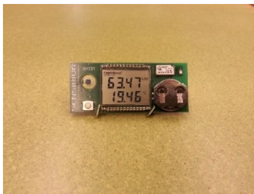
Figure 4.30: A Sensirion SHT31 hygrometer records the digital temperature and humidity of the outside ambient air.
