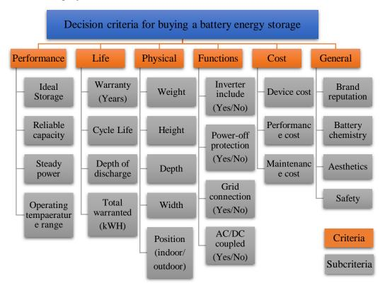
Figure 4: The identified attributes of energy storage technologies for multi-criteria analysis
