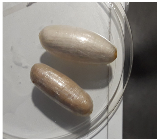
Figure 1. Sample of mechanically prepared pellets (length of 4–5 cm, diameter of 1.5–2 cm) (Courtesy: NT Tran).
