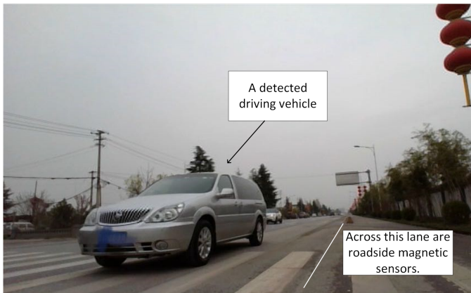
Fig. 11. A camera recorded driving scene of real experiments with magnetic sensors on the roadside.
