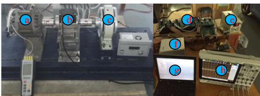
Fig. 15. Devices and platform for testing dynamic characteristics: (a) 16/10 pole SRM, (b) Torque and speed sensor, (c) Magnetic powder brake, (d) Power converter and drive circuit, (e) Power supply, (f) dSPACE, (g) PC, and (h) Oscilloscope.
