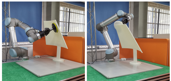
Fig. 4. Example configurations to cover the blade’s concave and convex sides.
