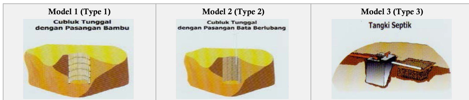
Figure 6: Variations in toilet model underground bottom section
