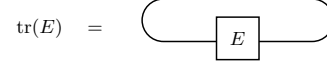
Fig. 3. The tensor network of computing the trace of the functionality matrix E of a (noiseless or noisy) circuit.
