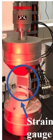
FIGURE 4.7: Testing strain gauge using Instron E10000 machine [5].
