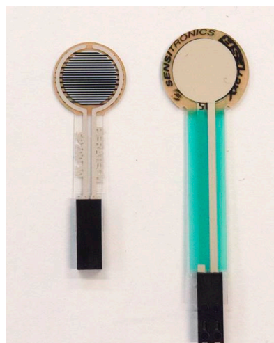
Figure 1. Piezoresistive force sensors used for evaluation: (left) Peratech QTC TM ; (right) Sensitronics ® FSR.
