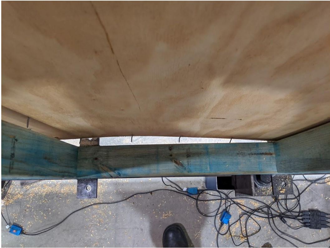
Figure 19: Test Panel M1.3 After Failure showing Nail Pullout Failures.
