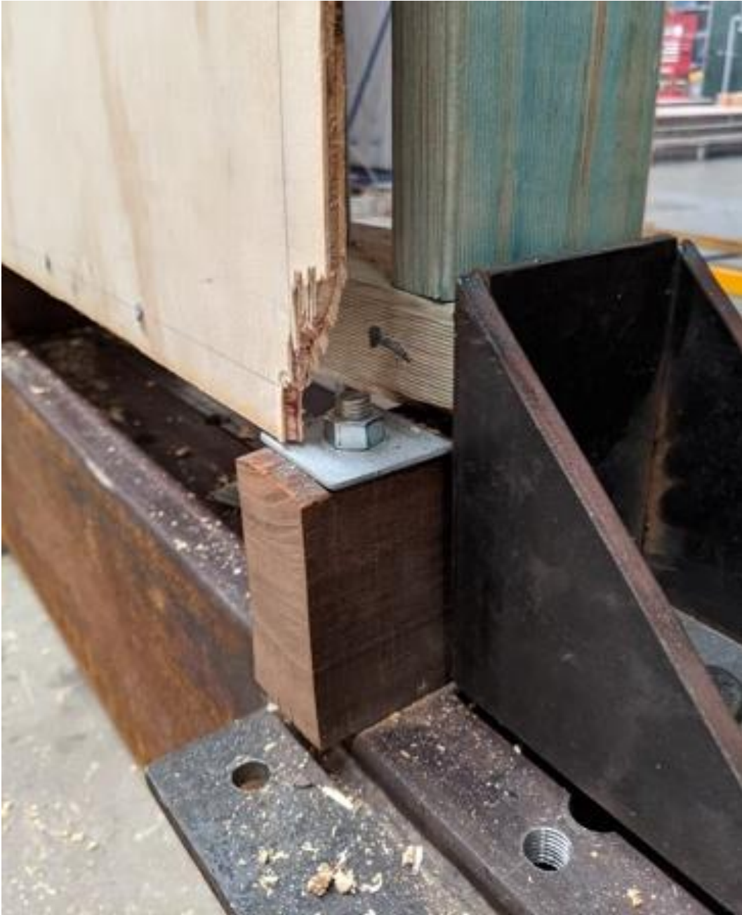
Figure 20: Test Panel C4.2 After Failure.
