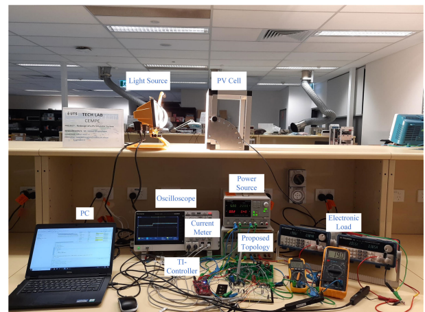
FIGURE 6. Experimental setup for the proposed PV emulator.
