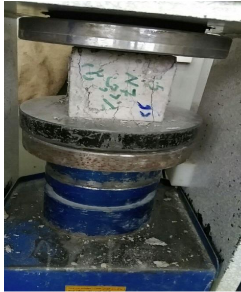
Figure 3. A cubic sample during the compressive strength test.
