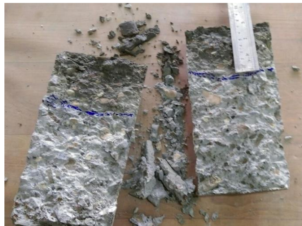
Figure 5. Measuring water penetration in the cylindrical sample.
