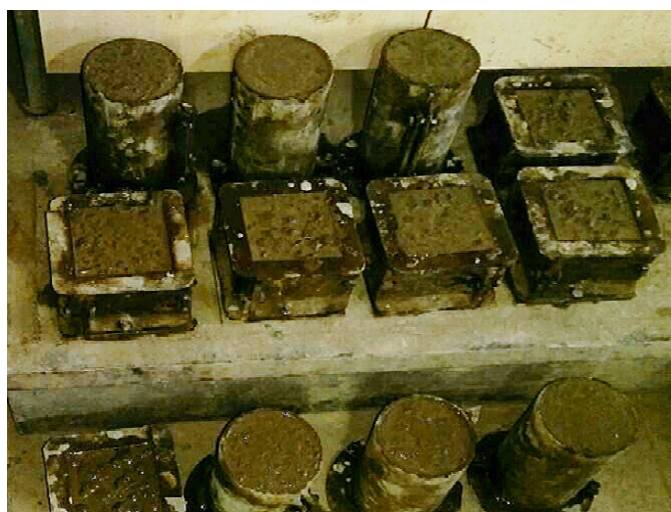
Figure 1. Fresh concrete in cubic and cylindrical molds.
