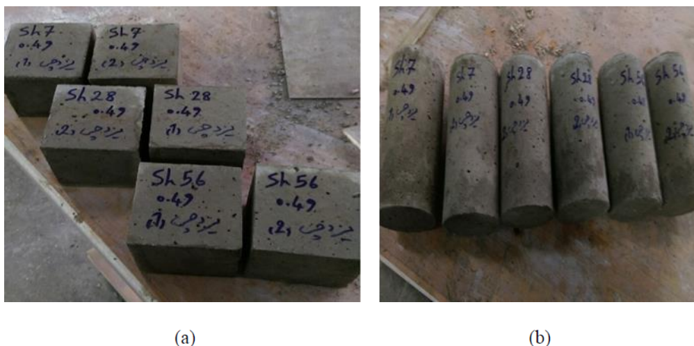
Figure 2. Concrete samples: (a) cubic samples, (b) cylindrical samples.
