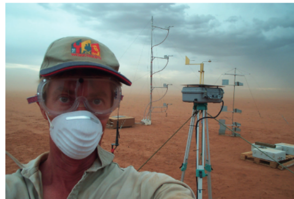
Figure 7: Citizen scientists in the DustWatch program monitor dust activity using instruments such as deposition traps and high volume air samplers. OEH/Simone Cottrell
