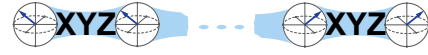
(b) The nearest-neighbour Heisenberg model is a chain of N qubits with XYZ coupling between each neighbouring qubits.
