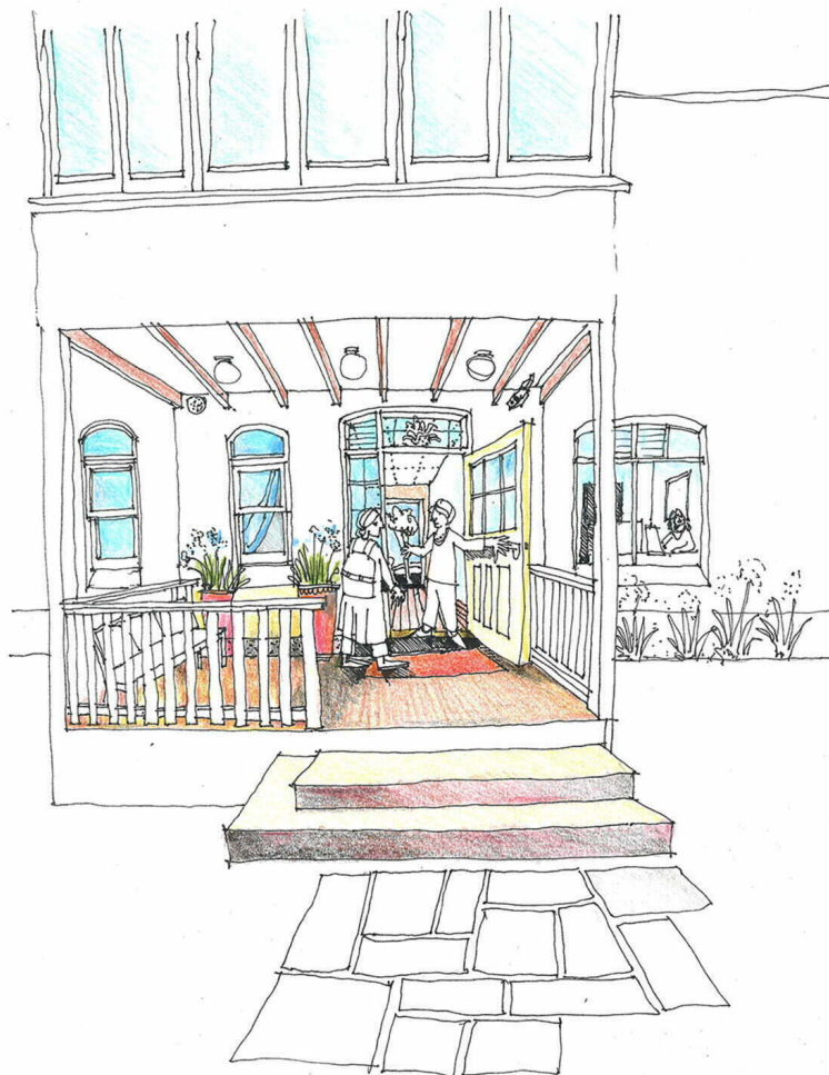
A layered entry sequence with security gates, entry gate and front door screen to enable controlled access of visitors/strangers. Secure screens to doors and windows for actual and perceived safety.
