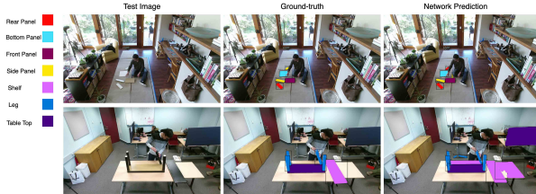
Figure 5: Illustration of part instance segmentation failure cases. (Top row) Mask R-CNN fails to correctly classify different panels of the drawer due to high similarity. (Bottom row) Mask R-CNN incorrectly segments part of the working surface as a furniture part (e.g., shelf) leading to considerable false positives.
