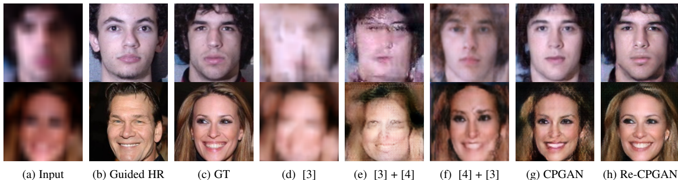
Fig. 2: Comparison of our proposed Re-CPGAN with the state-of-the-art methods ( 16 \times 16, 8\times ) 1 . (a) Interpolated unaligned NI-LR image. (b) Guided UI-HR image ( 128 \times 128 pixels). (c) Ground-truth UI-HR image ( 128 \times 128 pixels, not available in training ). (d) Illumination normalization result of (a) by applying [3]. (e) Face hallucination result of (d) by applying [4]. (f) Result of face hallucination followed by illumination normalization by applying [4] and then [3] to the NI-LR face. (g) Result of our previous method CPGAN [5]. (h) Result of Re-CPGAN ( 128 \times 128 pixels).
