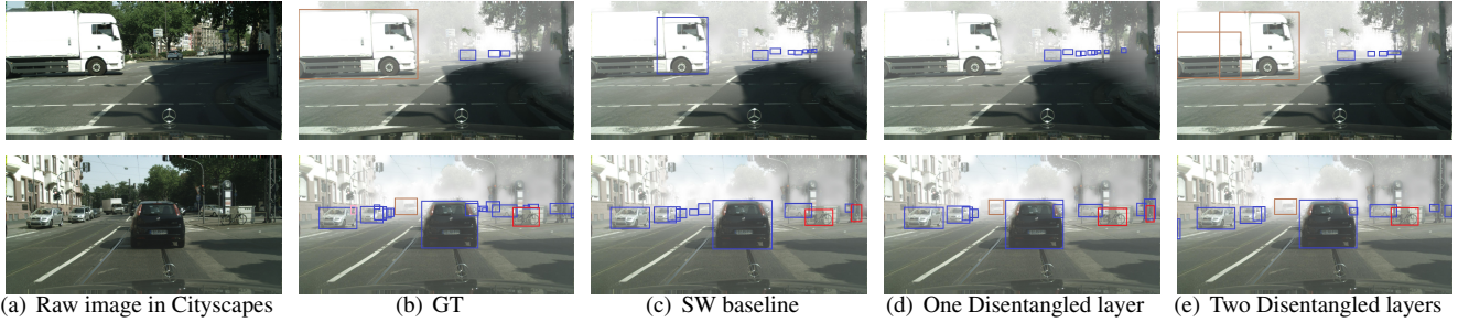
Figure 5. Detection results on the “Cityscapes \rightarrow FoggyCityscapes” scene. ‘GT’ indicates the groundtruth result. ‘One Disentangled layer’ denotes we only use the second disentangled layer in the model. We can see that our method, i.e., using two disentangled layers, could locate and recognize objects existing in the two foggy images accurately, e.g., the truck , car , and bicycle .
