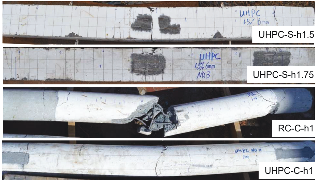
Fig. 3.5. Column failure patterns
