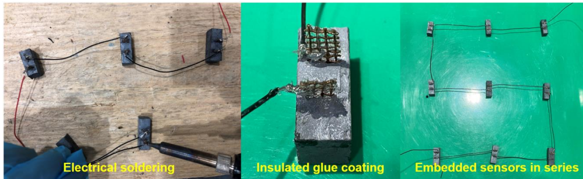
Figure 8.10. The joint connection, insulated glue coating and final cement-based sensors in series
