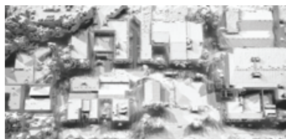
Fig. 06.02.01 [Top] Canopy cover extraction, and [Bottom] shadow analysis, produced from textured 3D photogrammetry data. Source: Author
