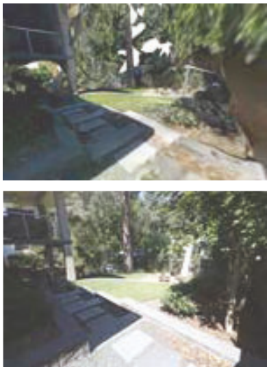
Fig. 10.02.01 Fig. 10.02.01 The 3D model [top] was aligned with a real-world camera angle [bottom] to compare real vs simulated shadow cast, for validation of the methodology.
