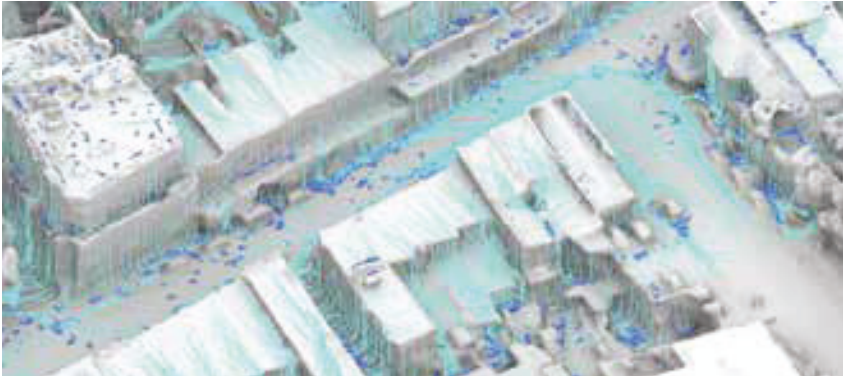
Fig. 07.02.04 Water flow-line simulations across the three example sites in Willoughby, using Grasshopper functionality and 3D point-cloud derived meshes.
