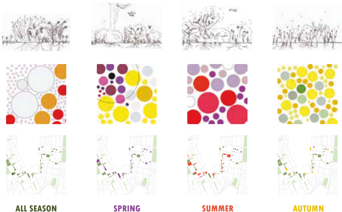
Fig. 03.05.02 Seasonal gardens were located on rooftops, based on simulated sun exposure potential during their flowering period. Source: The Green Ribbon, Author.
