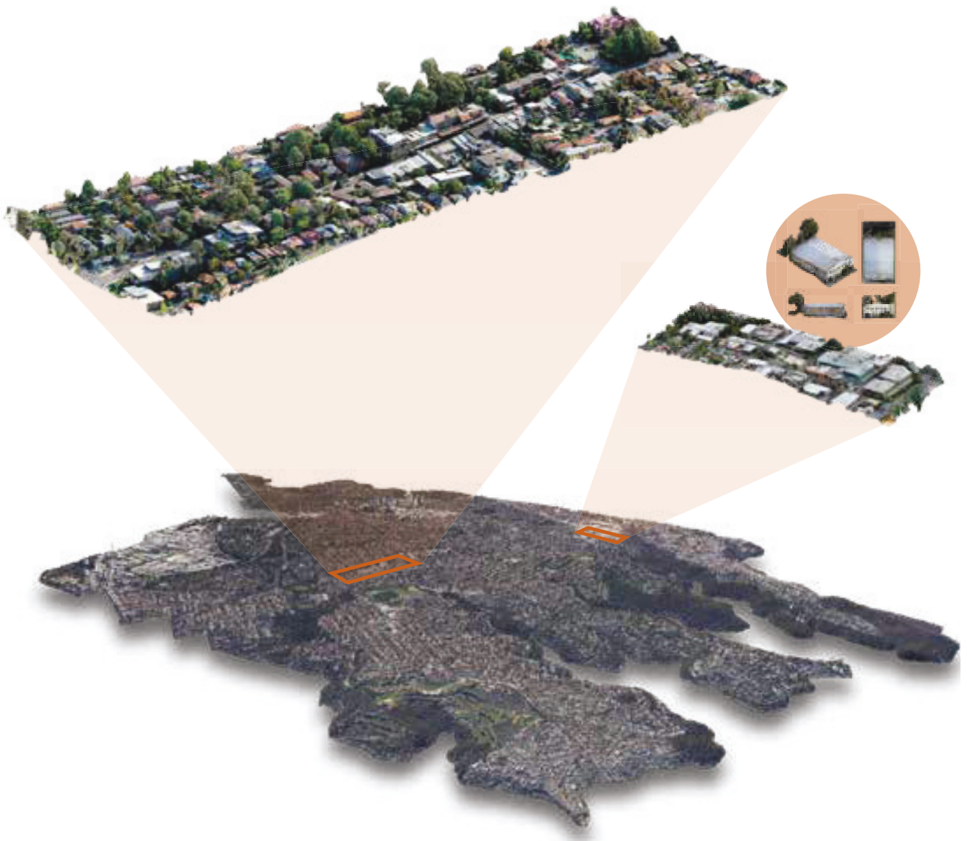
Fig. 06.02.02 Point Cloud Data of Willoughby LGA, hybridised with finer-grain photogrammetry data of Willoughby Rd and High St. Source: Author
