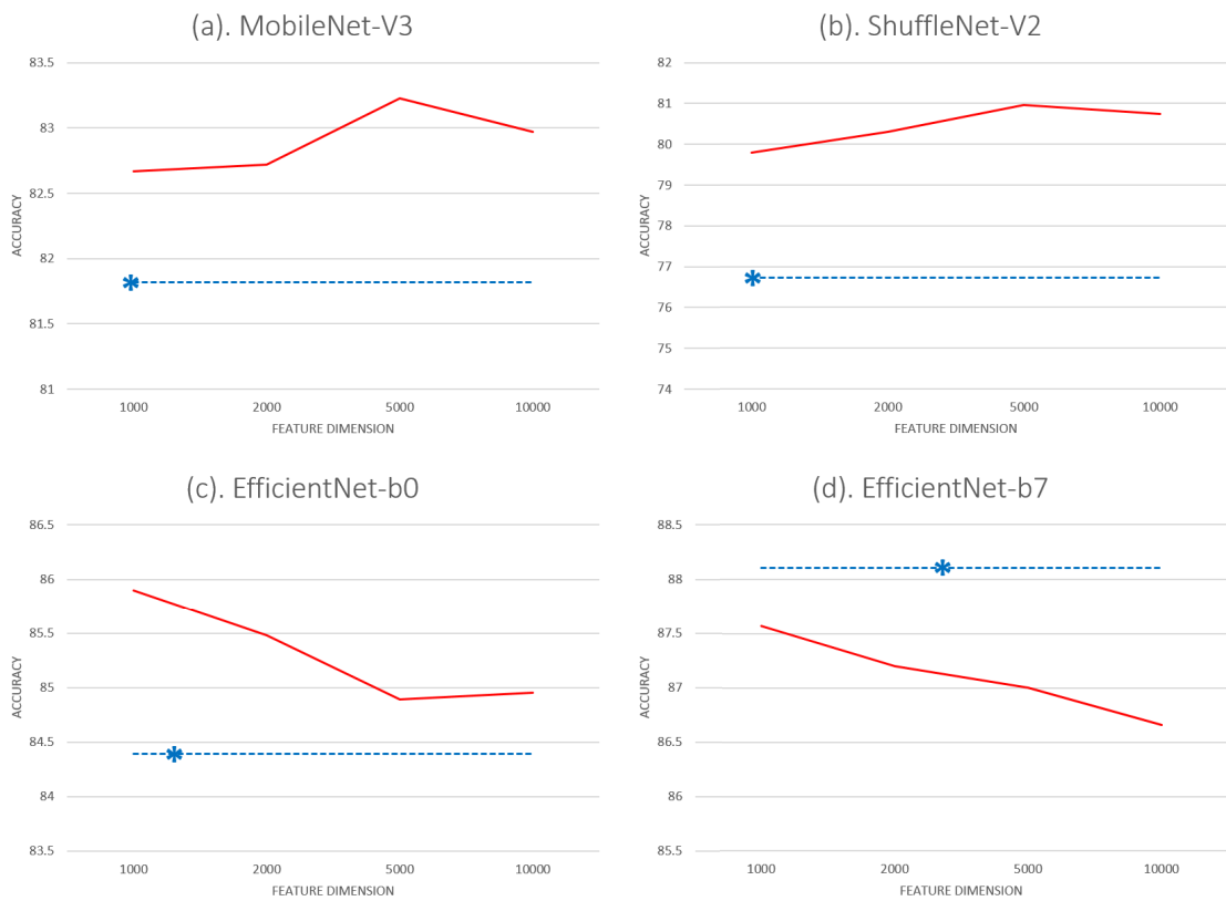
Figure 7.1: The CUB-200-2011 prediction accuracy of SBP on four different backbones: (a). MobileNet-V3; (b). ShuffleNet-V3; (c). EfficientNet-b0; (d). EfficientNet-b7. The red lines indicate the accuracies using different feature dimension. The blue lines of dashes are the baseline of the original structures without SBP, and the blue stars is the feature dimension of the original structures.
