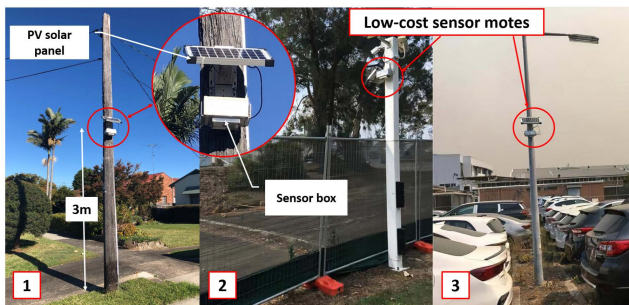
FIGURE 8. Sensor motes installed (1) T4 at a residential location, (2) T12 at the construction site, and (3) T2 in the car park.
