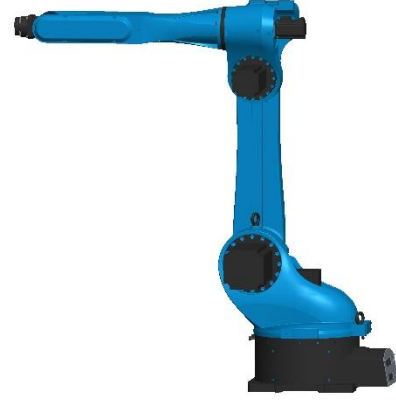
Fig. 12 Three-dimensional model of a six-axis industrial robot.
