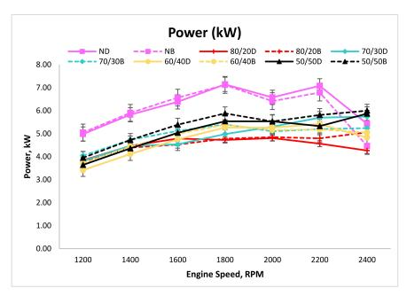
Figure 9. Power (kW) produced at various engine speed.
