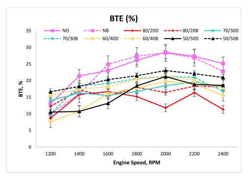
Figure 12. BTE percentage at various engine speed.
