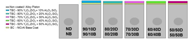
Figure 4. Piston crown configuration with specific coating mixture.
