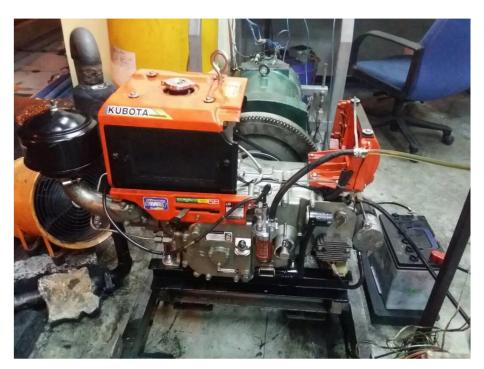
Figure 2. Kubota RT-125 diesel engine experimental setup.
