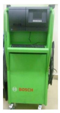
Figure 3. Photo of gas analyzer BOSCH BEA-150.
