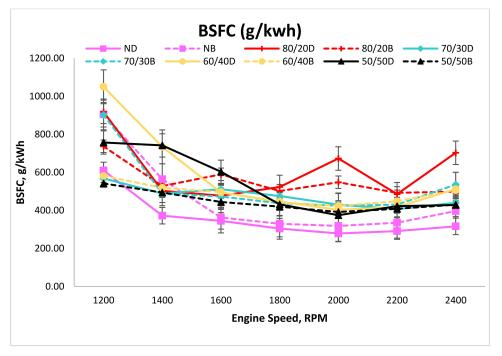
Figure 11. BSFC at various engine speed.
