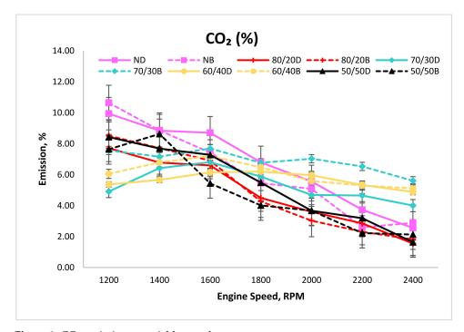
Figure 8. CO<sub>2</sub> emission at variable speed.
