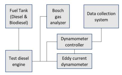
Figure 1. Schematic diagram for the experimental setup.
