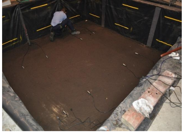
(b) Moisture sensors and pore pressure gauges
