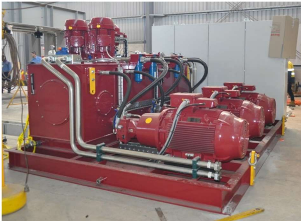
(c) Hydraulic power unit
