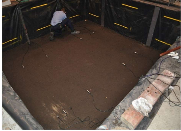
21 (b) Moisture sensors and pore pressure gauges
