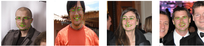
FIGURE 5. Visualized results of landmark detection using the proposed model. Red: predicted landmarks; Green: annotated landmarks
