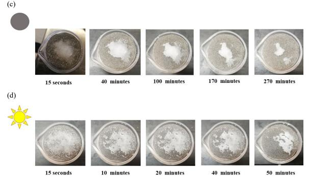
Fig. 10 Fig. 10 Self-cleaning properties of; PDA NWs-NF (a) in dark conditions (without sunlight), (b) under one sun intensity. Treated NF (c) in dark conditions (without sunlight), (d)
