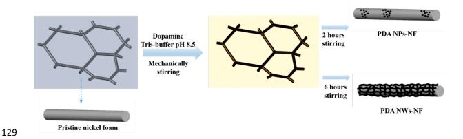
Fig. 1 Schematic of the fabrication process of PDA nanoparticles and PDA nanowires (NWs)on NF.
