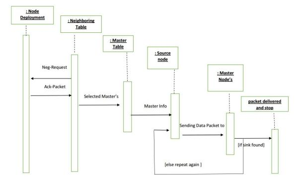
Figure 7. Sequence Diagram of ERPMSA-UWSN.
