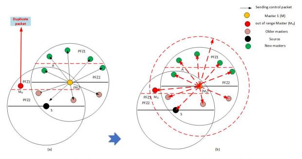
Figure 6. (a) Packet duplication (b) Master-Range extension to end data packet duplication.
