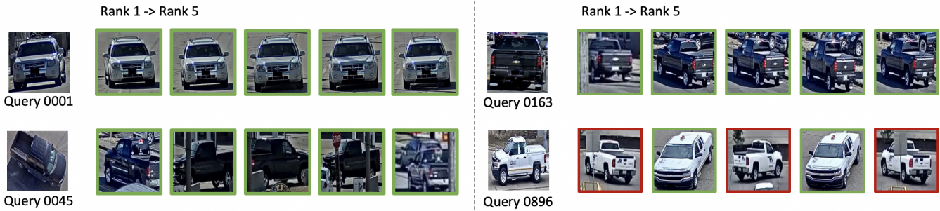
Fig. 6. Qualitative image search results using the vehicle query images from the CityFlow dataset. We select the four query images from different viewpoints, i.e. , the front view, the overhead view, the rear view and the side view. The results are sorted from left to right according to the similarity score. The true-matches are in green, when the false-matches are in red.
