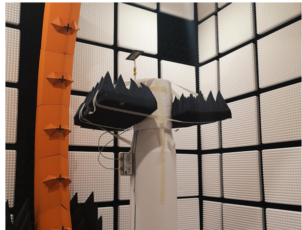
Fig. 15. Prototype quadrupole antenna as the antenna under test (AUT) in the anechoic chamber for measurement of its realized gain patterns and total efficiency.
