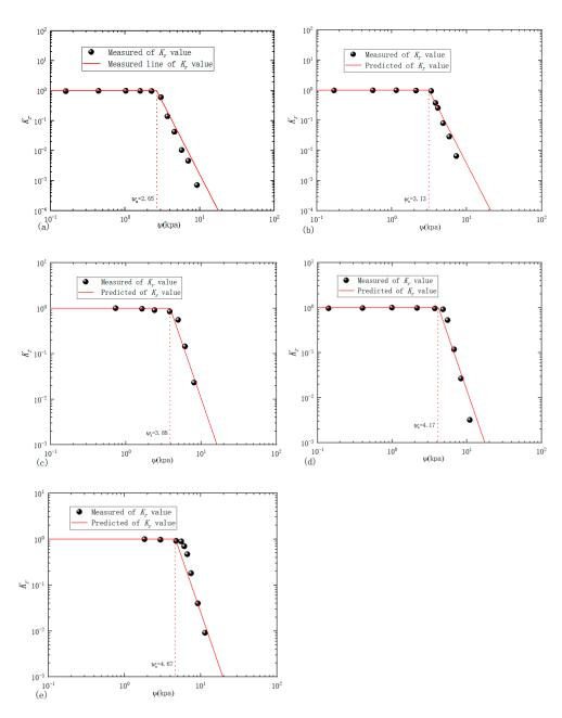
**Figure 5.** Prediction results of the unsaturated relative permeability coefficients of Columbia sandy loam with different void ratios: (**a**) e = 1.268; (**b**) e = 1.114; (**c**) e = 0.942; (**d**) e = 0.89; (**e**) e = 0.815.
