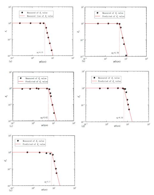
**Figure 4.** Touchet silt loam's different porosity ratio unsaturated relative permeability coefficient prediction results: (**a**) e = 1.012; (**b**) e = 0.916; (**c**) e = 0.815; (**d**) e = 0.733; (**e**) e = 0.653.
