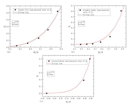
**Figure 3.** Fitting values of  $\lambda$  for three types of soil: (a) Touchet silt loam; (b) Columbia sandy loam; (c) unconsoildated sand.
