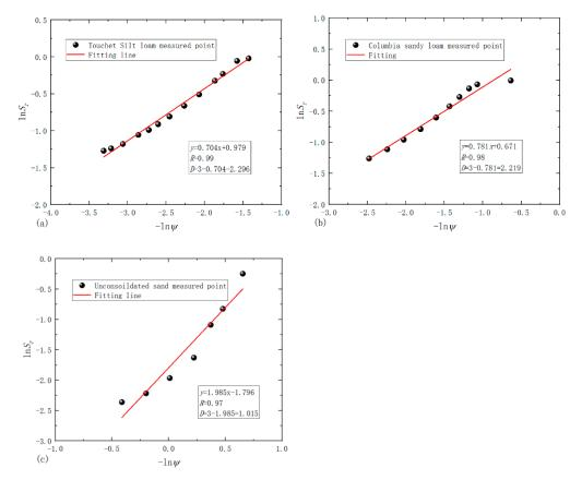
**Figure 2.** Fitting to obtain the fractal dimension of three soil types: (**a**) Touchet Silt loam; (**b**) Columbia sandy loam; (**c**) unconsoildated sand.
