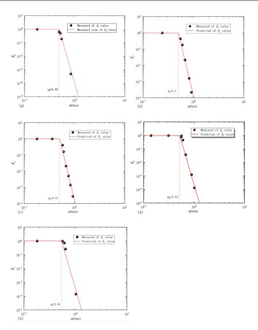
**Figure 6.** The prediction results of the unsaturated relative permeability coefficients of unconsoildated sand with different porosity ratios: (a) e = 0.852; (b) e = 0.825; (c) e = 0.799; (d) e = 0.767; (e) e = 0.715.
