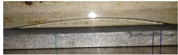
Figure 4: Deflection of the layers due to the rolling shape of the raw material
