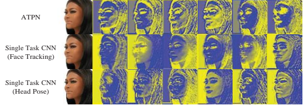
Figure 4: Column 1 shows the input image and column 2 to column 7 illustrate the low-level feature maps in the ATPN and two single task CNN.
