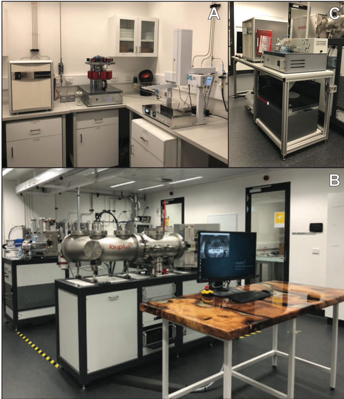
Figure 1: The Chronos ^{14}\text{C} Carbon-Cycle Facility at the University of New South Wales. Panel A: Elemental analyser with Carbonate Handling System 2 and Automated Graphitisation Equipment 3. Panel B: The Mini-Carbon Dating System with New Zealand ancient kauri workstation at the University of New South Wales. Panel C: Elemental analyser coupled to an isotope ratio mass spectrometer with the Gas Interface System.
