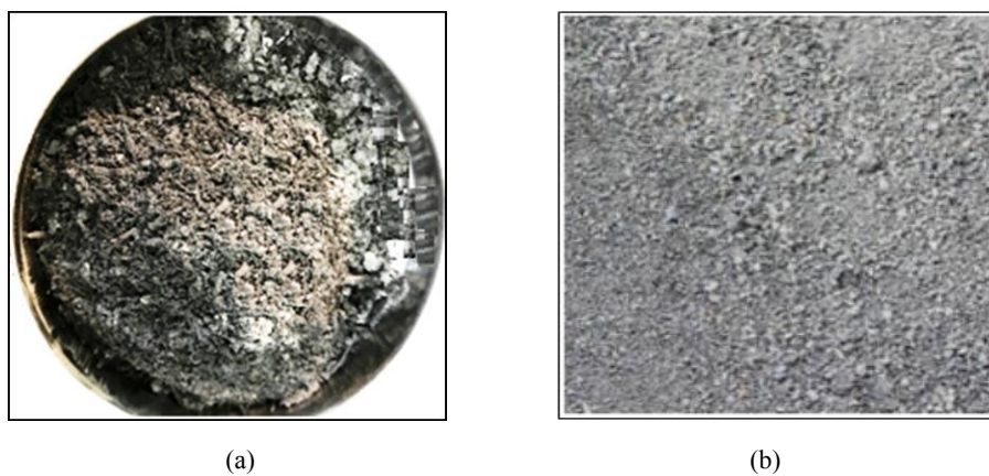
Figure 2. Photographic views of: (a) bagasse ash, and (b) stone dust
