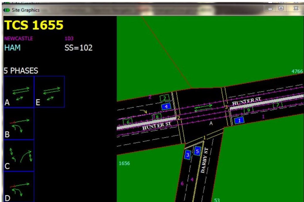
Figure 4.11 – Traffic signal phasing at the intersection of Hunter Street/Darby Street from SCATS data
