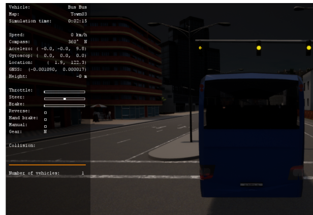
Fig. 9. Import the model into the CARLA simulator scene
