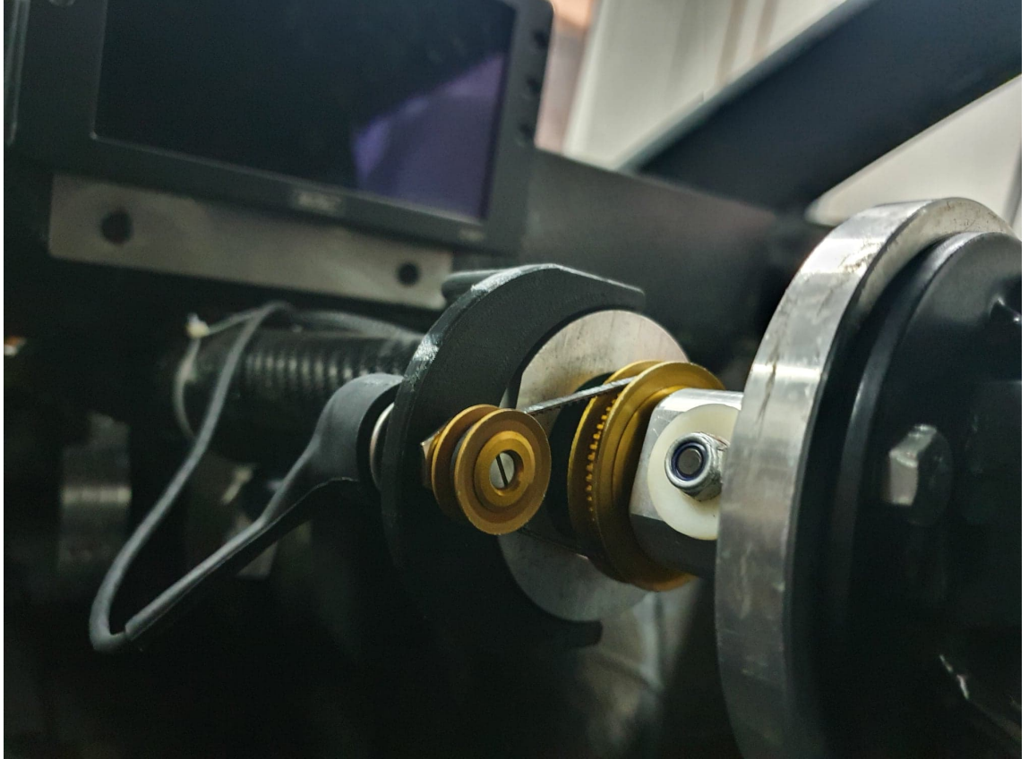
FIGURE 6.13: Steering angle sensor installed in the vehicle.
