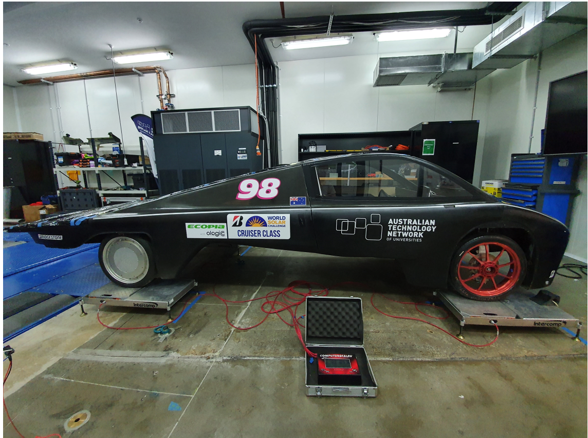
FIGURE 6.4: COG position measurement set-up
