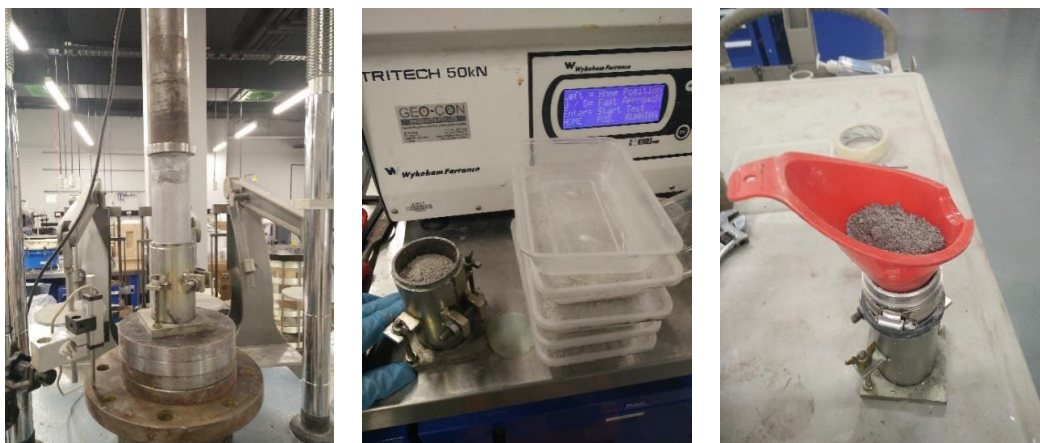
Figure 3.24 Snapshots of sample preparation for suction, bender element and triaxial tests
