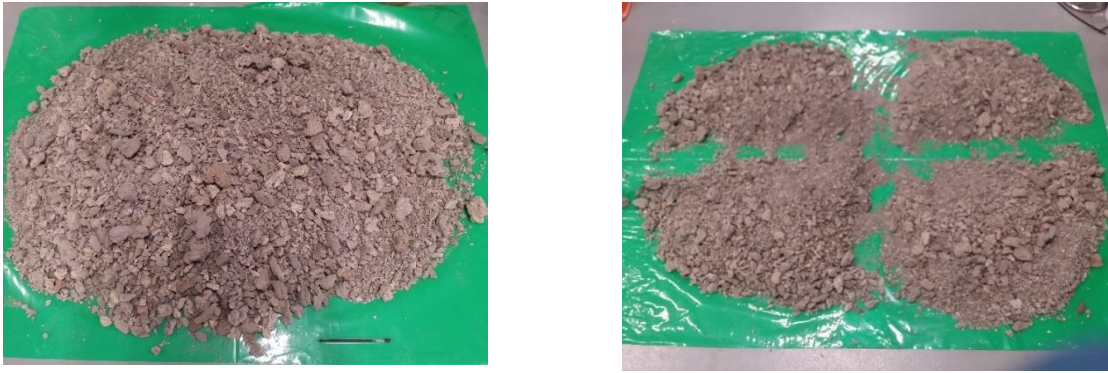
Figure 3.19 Quartering method for selecting representative samples of bottom ash
