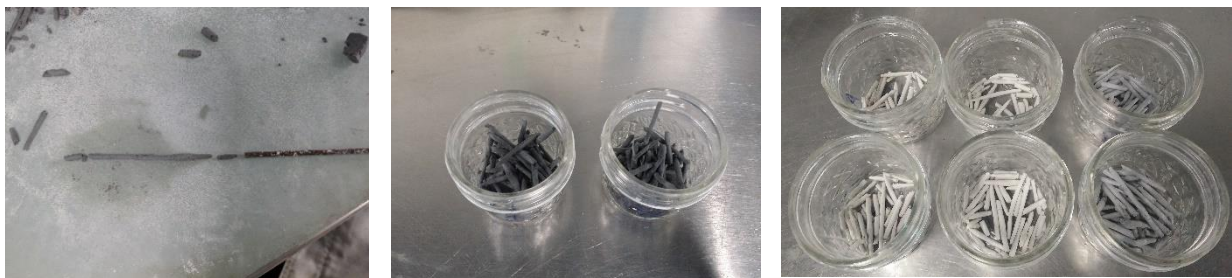
Figure 3.41 Plastic limit tests
