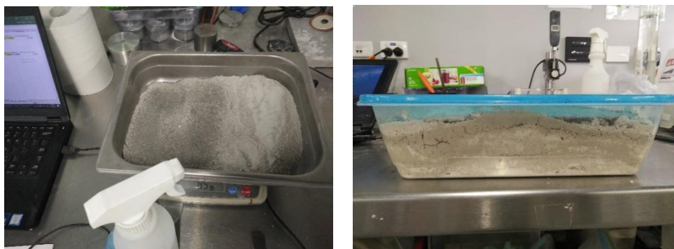
Figure 3.25 Moisturisation for treated soil samples
