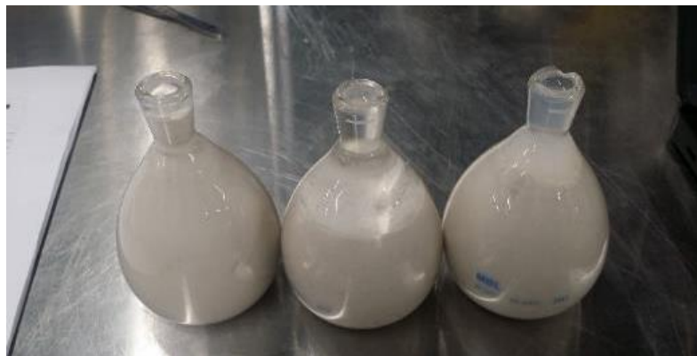
Figure 3.40 Three pycnometers for specific gravity tests
