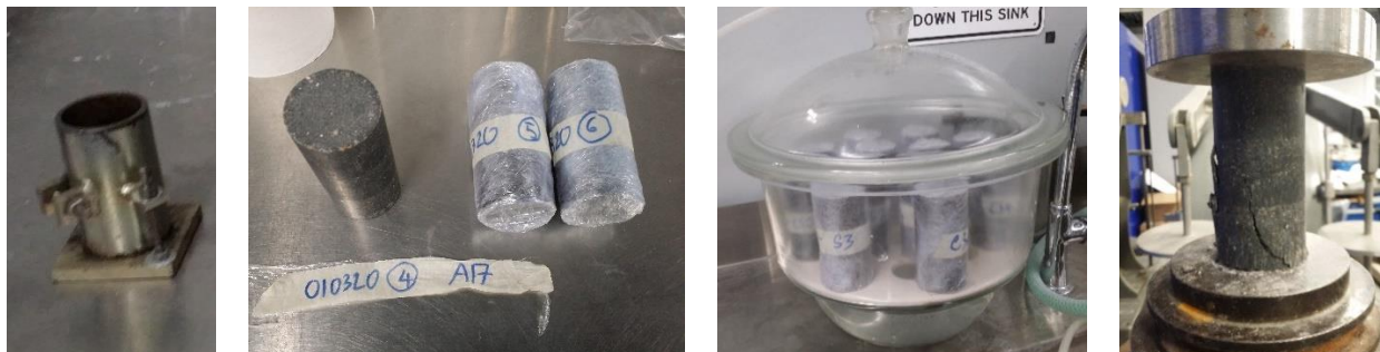
Figure 3.45 Unconfined compressive strength tests
