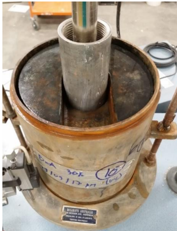
Figure 3.47 California bearing ratio test
