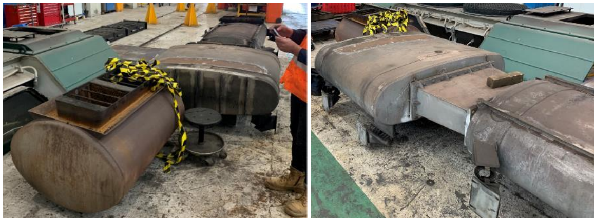
Figure 1 Comparison of crude older silencers, such as on the G Class (left - foreground) and larger coffin silencers such as from the 82 Class (background left, and foreground right). More recent locomotives such as NR, C44aci and GT46C ACe locomotives have even larger silencers than 82 Class.
