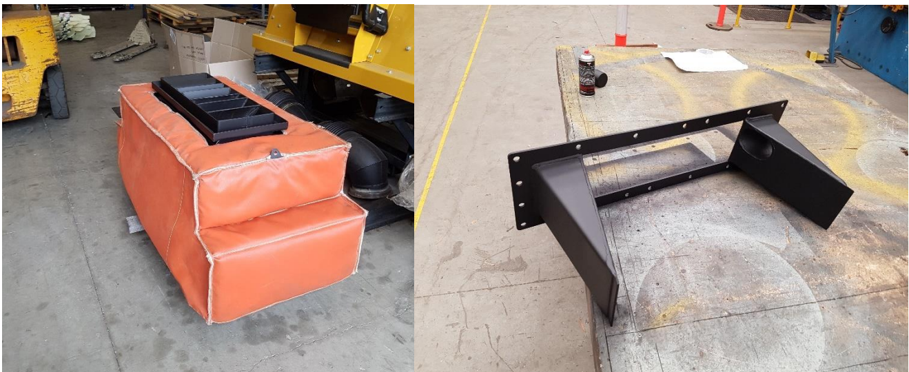
Figure 6 The completed silencer (left) with thermal blanket and flow transition device (right) ready for installation
