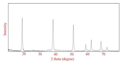
Fig. 2. XRD pattern of the Mg(OH)<sub>2</sub> nanoparticles
