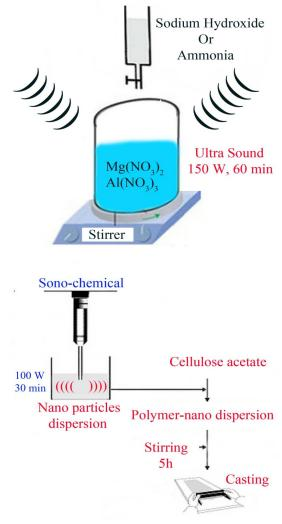
Fig. 1. Schematic of nanoparticle and nanocomposites preparation
