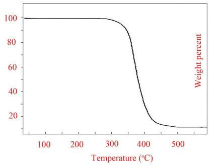
Fig. 7. TGA spectrum of the CA-Mg(OH), nanocomposite
