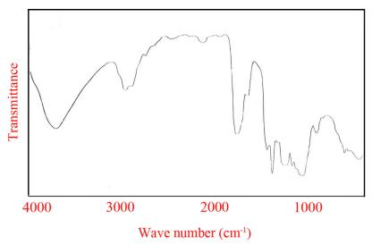
Fig. 6. FT-IR spectrum of the Mg(OH)<sub>2</sub> nanoparticles
