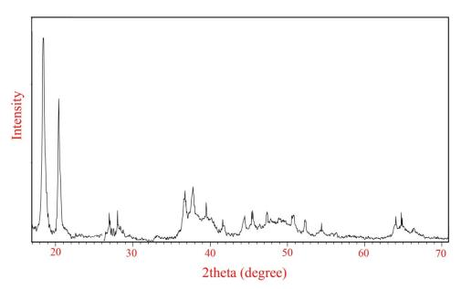
Fig. 3. XRD pattern of the Al(OH), nanoparticles
