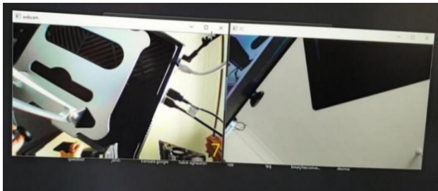
Figure 3: the two camera feeds. Camera feed of the gripper on the left shows the current position of the gripper claws.
