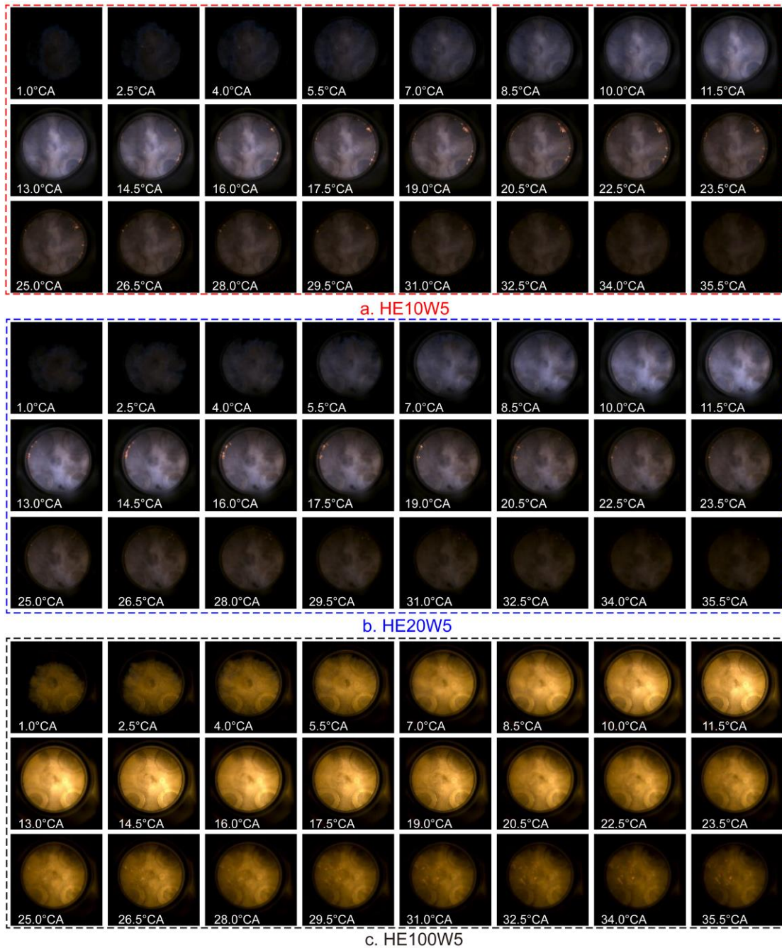
Figure 7. Flame development images for various test fuels ( n = 1200 r/min, indicated mean effective pressure (IMEP) = 0.4 MPa, injection timing: -280^\circ\text{CA} ) [106].
