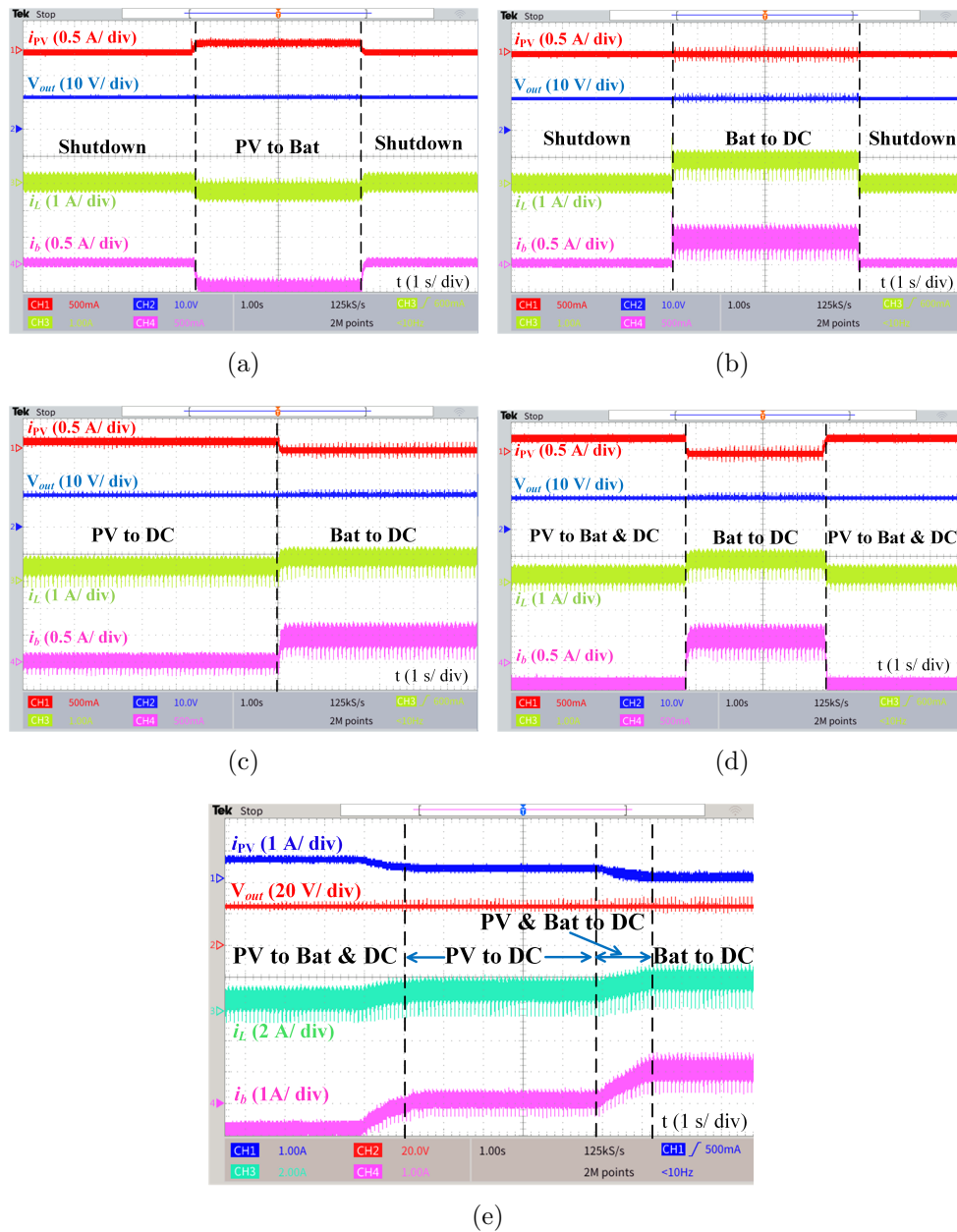
Fig 6.13: Waveforms of the transition between modes of the proposed converter.
