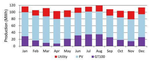
Figure 13. Monthly electric production of solar PV, GT100 and grid.
