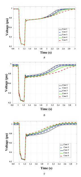
Fig. 4 Dynamic voltage profile at PCC for different cases (a) Phase A, (b) Phase B and, (c) Phase C
