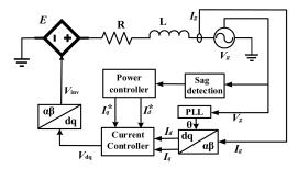
Fig. 2 Overall control structure of TL PV system
