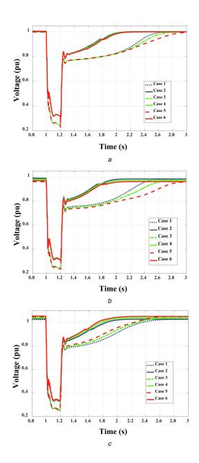
**Fig. 6** Dynamic voltage profile at PCC for (a) Phase A, (b) Phase B and, (c) Phase C
