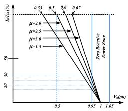
**Fig. 5** Reactive current injection with different values of  $\mu$
