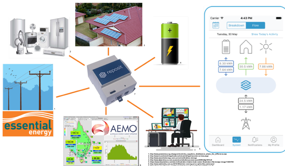
Figure 22. Essential Energy and Reposit Power’s control platform for NSW.
